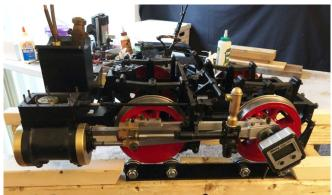
A few years back at White Creek, Larry Kepner showed me a valve gear setting trick he thought up. He mounted a piece of steel angle on the end of the crankpin and attached a magnetic digital angle finder used to set the angle of the blade of a table saw.
