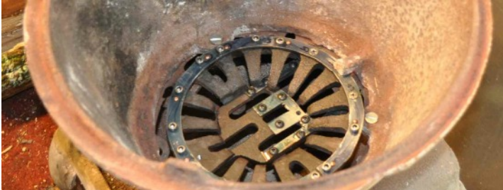
The Knox shop stove was out of commission because the cast iron pieces had cracked from long usage. After pricing new stoves and a lot of head scratching, Carl Schwab brazed the pieces together and is here checking the reconstructed grate.
