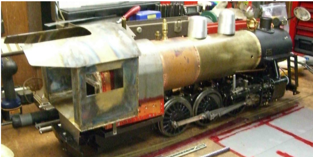
An updated view of the BLW's Narrow Gauge switcher with the rough cab in place
