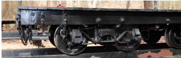
The new tender chassis showing Denis' nice detailing: oak platform boards, arch-bar trucks, stirrups and safety chains
