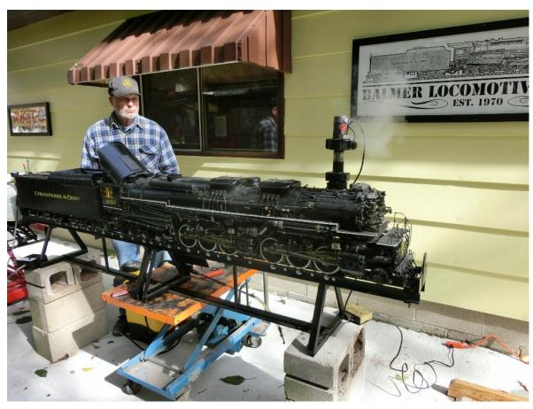
We got the Allegheny out and test fired it on our rolling stand and ran the engines on steam for the first time. The engines ran very well once we got them rolling and would stop and restart after that with no issue. We had a few of the accessories that worked like the air powered drain cocks and steam turbo generator.
