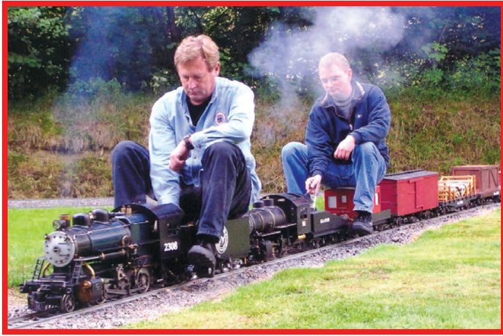
Double heading German style using a mogul and an 0-6-0 switcher. A very nice group of cars.
