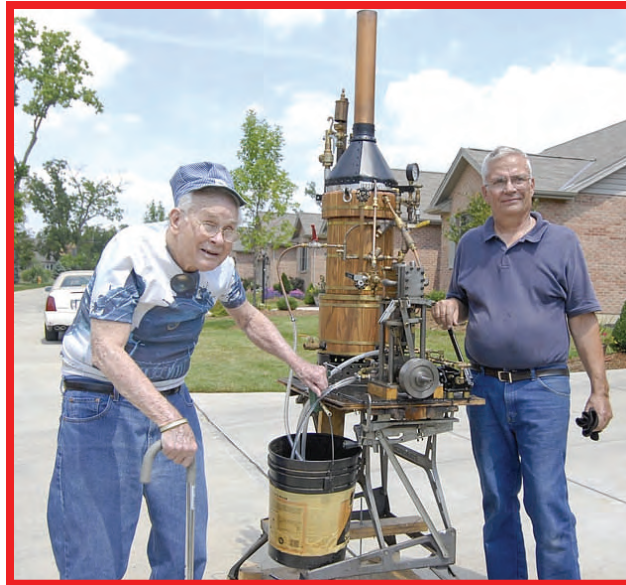
This is the heart of Carl's new boat—a vertical boiler and a single cylinder reversing engine. The whistle is something to hear and yes, it does work nicely. Now to get on with the rest of the boat.
