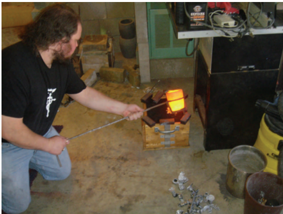
Chuck's son pouring Aluminum into a mold, completed castings on the floor
