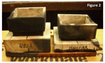
I made the molds and we tried to pour them with bronze. Due to the small cross section of parts, the molds did not fill before the metal froze. I changed the size of the pour
