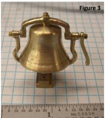
pouring the metal. This worked pretty well and there was only one small void in the bell that was easily repaired. (see figure 3)
