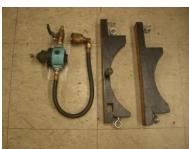
Valve with Fuel Line Coupler, Overflow Protection, Pressure-Relief Valve.
